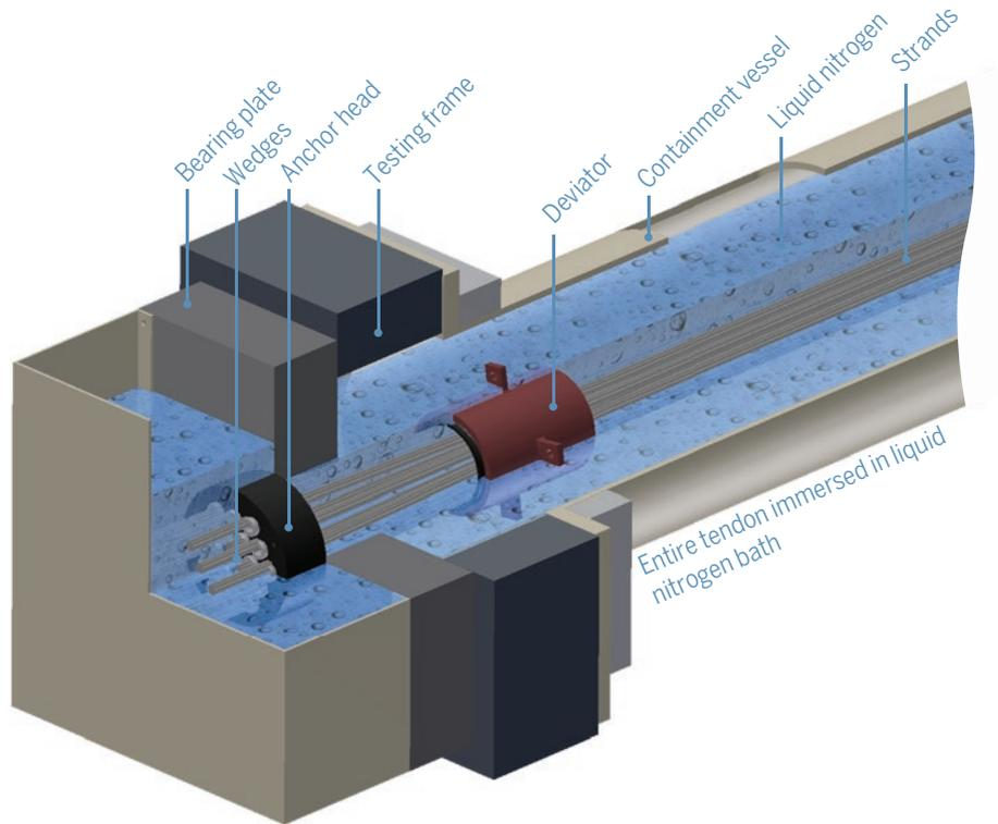
Thereby, the ultimate failure is always occurring at the tendon side under ambient temperature (see point A on graph), while at this load level the tendon part, which is immersed into the liquid nitrogen bath, is still in the linear elastic zone (see point B).
