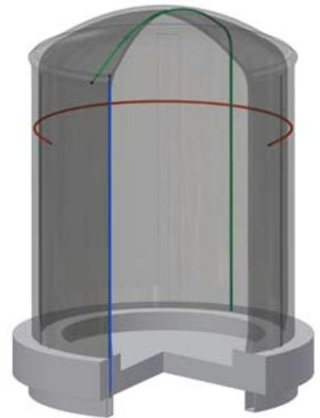
force can be monitored by lift-off tests or through permanently installed equipment. They can be retensioned and they can also be removed for visual inspection and eventually replaced.
