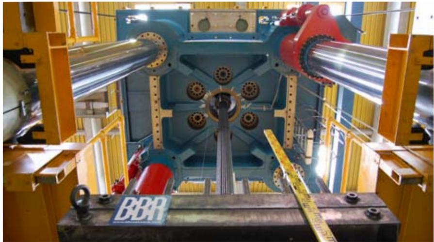
Although well in excess of the ETAG requirements, the team decided to go above eight million load cycles – already over four times more than required – in one additional voluntary test run. It was amazing that, even under these extremely hard conditions, the tendon endured this gruelling fatigue testing without any strands breaking.
