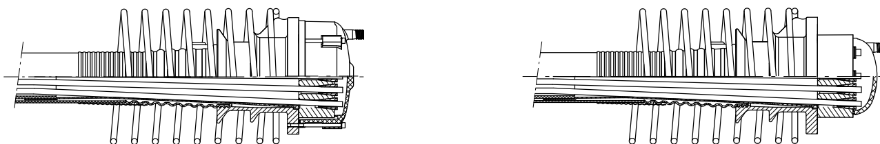
Stressing anchorage, accessible fixed anchorage, replaceable SAR, FAR 1), 2) With bare strands or monostrands
